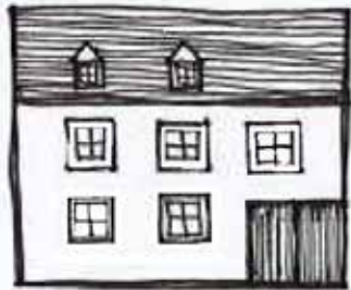
Loft conversion incorporating gabled dormers.
