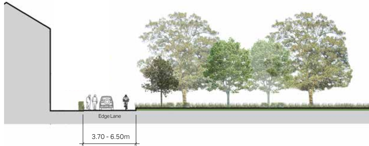
Figure 110: Cross-section to illustrate some dimensions for edge lanes.
