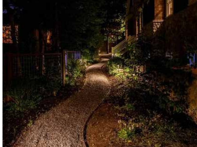
Figure 200: Example of path lighting where all lights are directed downwards, whilst the light sources are obscured.
