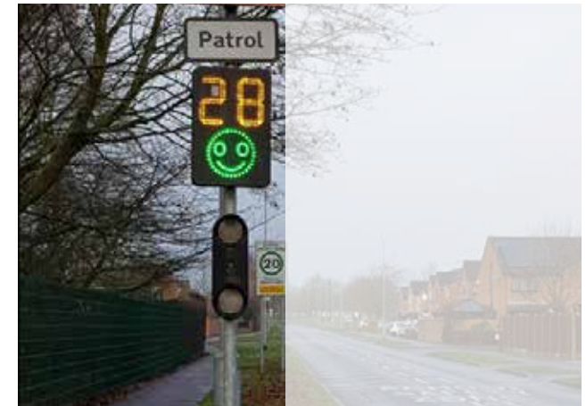
Figure 106: Example of an interactive signage to indicate speed limits within a residential area, elsewhere in UK.
