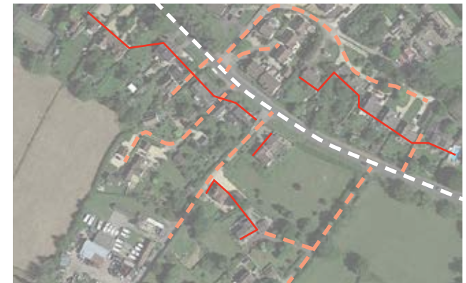
Figure 90: Aerial view of pattern of private drives and cul-de-sacs (orange dotted line) with irregular building lines (red line), set back from the main road (white dotted line) in Shaw
